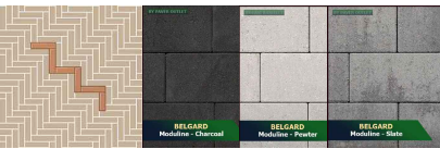
ENTRY WALK | PAVER MAINFIELD | TOTAL AREA 3,121 sf MFR: MODULINE - BELGARD. THICKNESS: 2-3/8". RECTANGULAR PLANK 4x12
